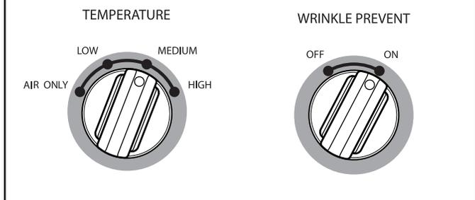
Select temperature and options by turning the knob to the desired position or select the Automatic Dry Cycle that has the temperature included in the cycle selections.
