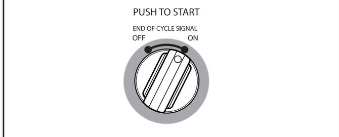
Turn the END OF CYCLE SIGNAL knob to select the desired setting (On or Off). The End of Cycle Signal produces an audible sound when the drying cycle is finished. Promptly removing clothes at the end of the cycle reduces wrinkling.
