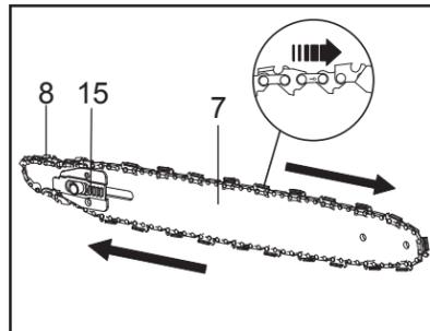
4. Check to make sure all parts are seated properly and hold chain and guide bar in a level position. (See Fig. 4c)
