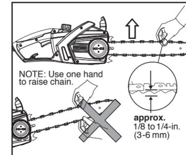
**NOTE:** If chain tension does loosen in the course of chain saw use, retension the chain as follows: Loosen the Chain Tension knob by turning it counterclockwise 3 full turns. Make sure that the cover plate is securely tightened in place. Proceed to tension chain by performing steps 1 - 3 listed above.
