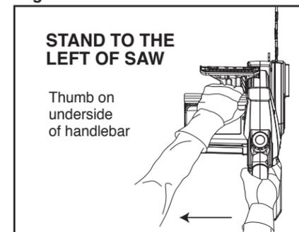
Use the chain saw only with secure footing. Hold the chain saw at the right-hand side of your body. **(See Figs. 11 and 12)**
