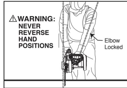
1. A good, firm grip on the saw with both hands will help you maintain control. Don't let go. Grip the rear handle with your right hand whether you are right or left handed. Wrap the fingers of your left hand over and around the front handlebar, and your left thumb under the front handlebar. Keep your left arm straight with the elbow locked.
