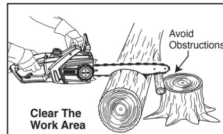
1. **KICKBACK** is the backward, upward or sudden forward motion of the guide bar occurring when the saw chain near the upper tip of the guide bar contacts any object such as a log or branch, or when the wood closes in and pinches chain in the cut. Contacting a foreign object in the wood can also result in loss of chain saw control.
