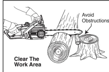
**KICKBACK** is the backward, upward or sudden forward motion of the guide bar occurring when the saw chain near the upper tip of the guide bar contacts any object such as a log or branch, or when the wood closes in and pinches chain in the cut. Contacting a foreign object in the wood can also result in loss of chain saw control.
