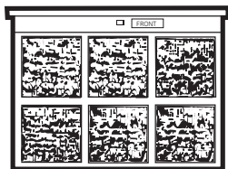
Dirty filter— Needs cleaning
