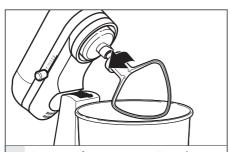
Remove the accessory: Turn the speed control to "0", unplug the Stand Mixer, and tilt the motor head 2 back; then, press the accessory upward as far as possible, turn the accessory clockwise and pull it away from the beater shaft.
