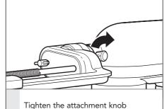
by turning it clockwise until the attachment is completely secured 4 to the Stand Mixer. See the Instructions manual that came with your attachment for detailed directions on using the attachment.
