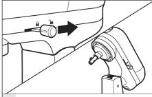
Raise the motor head: Slide the locking lever to the unlock position and lift the motor head. Once lifted, slide the locking lever to the lock position to keep the motor head up.
