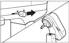
Raise the motor head: Check to be sure that the Stand Mixer is unplugged, and the speed control is turned to "0"; then slide the locking lever to the unlock position and lift the motor head. Once lifted, slide the locking lever to the lock position to keep the motor head up.
