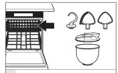
The bowl, flat beater, dough hook, Flex Edge beater, and pouring shield\* may be washed in a dishwasher (top 2 shelf only); or, clean them thoroughly in hot, sudsy water and rinse completely before drying. Do not store beaters on the shaft.
