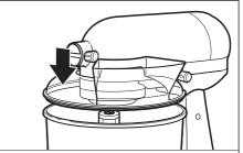
(OPTIONAL) Place the pouring shield\*: Slide the pouring shield\* from the front of the Stand Mixer over the bowl until the pouring shield\* is centered. The bottom rim of the pouring shield\* fits inside of the bowl. The pouring chute will be just to the right of the attachment hub as you face the Stand Mixer.
