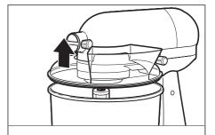
(OPTIONAL) Remove the pouring shield\*: Lift the front of the pouring shield\* clear of the rim of the bowl. and pull away from the Stand Mixer.
