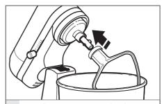
Attach any accessory: Slip the accessory onto the beater shaft and press upward as far as possible. Turn the accessory counterclockwise to hook the accessory over the pin on the shaft.
