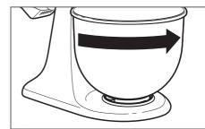
Remove the bowl: Gently turn 3 the bowl counterclockwise to release it from the bowl clamping plate.
