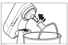
Attach any accessory: Slip the accessory onto the beater shaft and press upward as far as possible. Turn the accessory counterclockwise to hook the accessory over the pin on the shaft.
