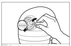
Turn the attachment knob counterclockwise to remove attachment hub cover.
