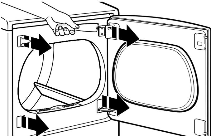
3. Using a T20<sup>®</sup> screwdriver, remove screws (A) and then screws (B) from each of the 2 hinges attaching the dryer door to the front panel of the dryer. Set the hinge screws off to the side for use in reinstalling the door.
