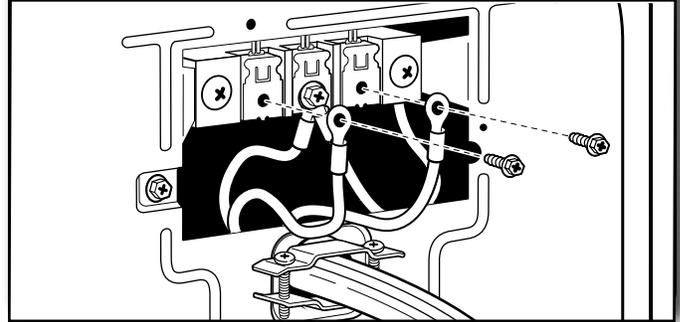
Connect remaining wires to outer terminal block screws. Tighten screws.
