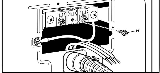
Remove center terminal block screw (B).
