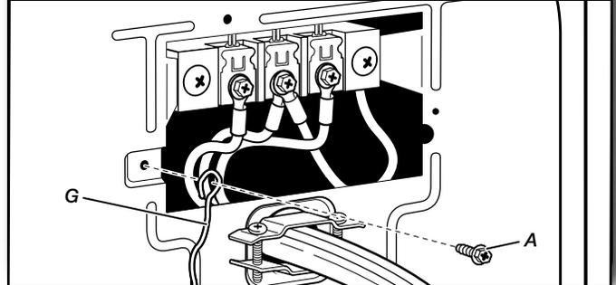
Connect a separate copper ground wire (G) from the external ground conductor screw (A) to an adequate ground. Finally, reinsert tab of terminal block cover into slot of dryer rear panel. Secure cover with hold-down screw. Now, go to "Venting Requirements."
