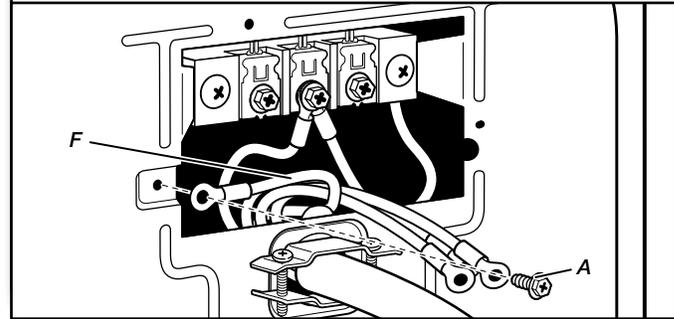
Connect ground wire (F) (green or bare) of power supply cord to external ground conductor screw (A). Tighten screw.
