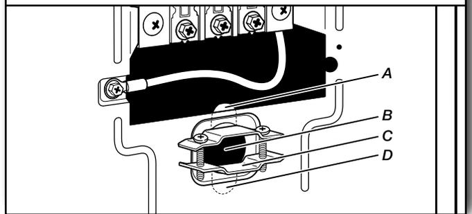
Remove the screws from a 3/4" (19 mm) UL listed strain relief (UL marking on strain relief). Put the tabs of the two clamp sections (C) into the hole below the terminal block opening (B) so that one tab is pointing up (A) and the other is pointing down (D), and hold in place. Tighten strain relief screws just enough to hold the two clamp sections (C) together.
