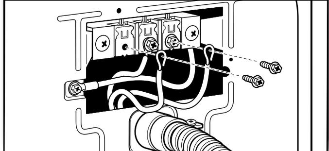
Place hooked ends of remaining direct wire cable wires under outer terminal block screws (hooks facing right). Squeeze hooked ends together and tighten screws. Finally, reinsert tab of terminal block cover into slot of dryer rear panel. Secure cover with hold-down screw. Now, go to "Venting Requirements."
