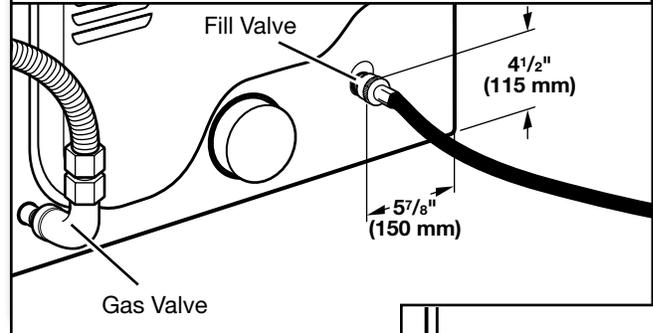
Attach other end of long hose to fill valve at bottom of dryer back panel. Screw on coupling by hand until it is seated on fill valve connector. Using pliers, tighten the couplings an additional two-thirds turn.
