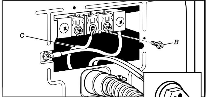
Place hooked end of neutral wire (white or center) (C) of direct wire cable under center terminal block screw (B). Squeeze hooked end together. Tighten screw.
