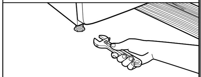
If dryer is not level, prop up using a wood block. Use wrench to adjust legs up or down, and check again for levelness.
