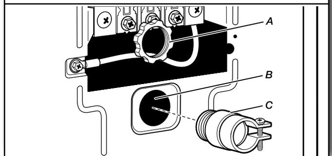
Unscrew the removable conduit connector (A) and any screws from a 3/4" (19 mm) UL listed strain relief (UL marking
