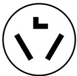
Power supply cord 3-wire receptacle (NEMA Type 10-30R):
