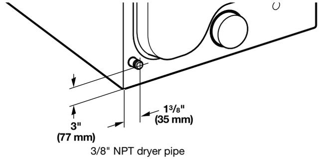
**NOTE:** For a garage installation, the gas pipe height must be an additional 18" (460 mm) from the floor.
