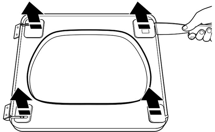
6. Using a #2 Phillips screwdriver, remove the remaining 4 screws from the hinges. Then remove hinges A and B and set both the screws and hinges aside.
