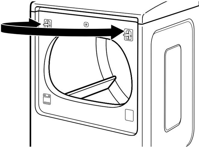
3. Install 2 plastic covers from the accessory kit into the spaces where the hinges were removed. Place the plastic hinge covers over the exposed hinges.
