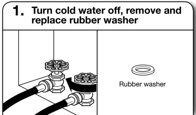
Turn cold water faucet off and remove washer inlet hose. Remove old rubber washer from inlet hose and replace with new rubber washer.
