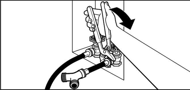
Using pliers, tighten the couplings with additional two-thirds turn.
