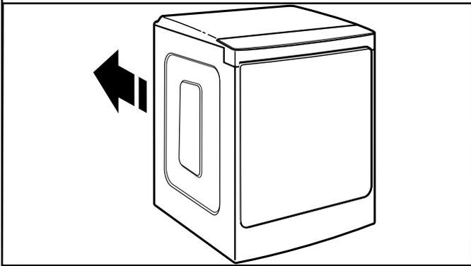
Move dryer to final location. Avoid crushing or kinking vent.
