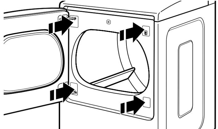
2. Hang the door on the unit by placing set pin in dryer cabinet hole and sliding door down. Using a Phillips screwdriver, install screws 1 and 3 and then screws 2 and 4. Tighten all hinge screws.
