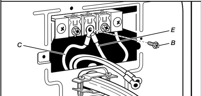
Connect neutral ground wire (E) and neutral wire (white or center wire) (C) of power supply cord or cable under center terminal block screw (B). Tighten screw.
