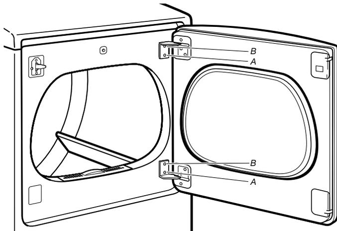
4. Remove the dryer door from the cabinet by lifting upward and out. Lay the door on a towel or a soft cloth you placed on a flat workspace.
