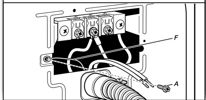
Connect ground wire (green or bare) (F) of direct wire cable to external ground conductor screw (A). Tighten screw.
