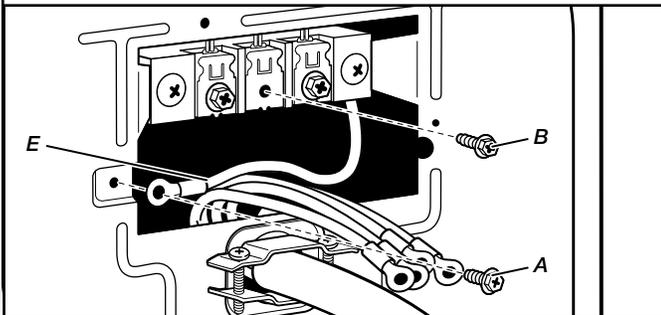
Remove center terminal block screw (B). Remove neutral ground wire (E) from external ground conductor screw (A). Reinstall ground conductor screw (A).
