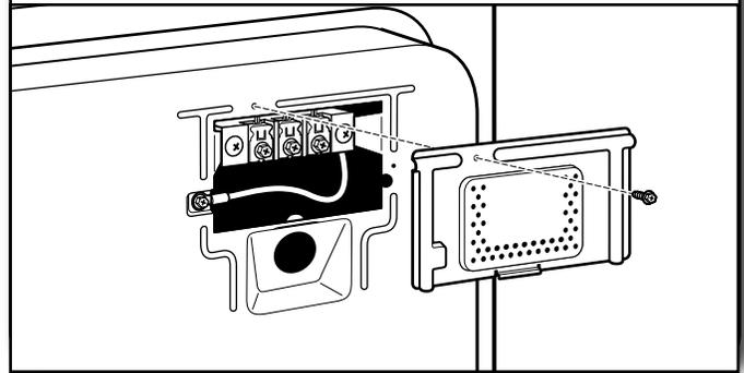
Remove hold-down screw and terminal block cover.
