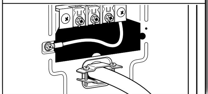
Put power supply cord through the strain relief. Be sure that the wire insulation on the power supply cord is inside the strain relief. The strain relief should have a tight fit with the dryer cabinet and be in a horizontal position. Do not further tighten strain relief screws at this point.
