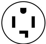
Power supply cord 4-wire receptacle (NEMA Type 14-30R):
