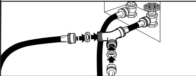
Attach dryer 5 ft (1.5 m) inlet hose ends to the "Y" connector. Attach washer cold inlet hose to other side of "Y" connector. Screw on coupling by hand until it is seated on connector. Using pliers, tighten the couplings an additional two-thirds turn.
