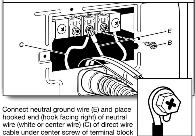
Connect neutral ground wire (E) and place hooked end (hook facing right) of neutral wire (white or center wire) (C) of direct wire cable under center screw of terminal block (B). Squeeze hooked ends together and tighten screw.
