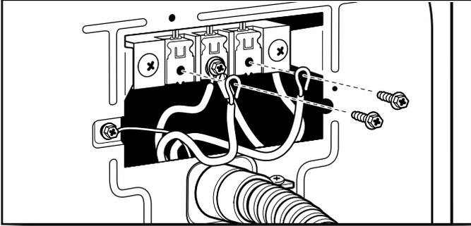
Place hooked ends of remaining direct wire cable wires under outer terminal block screws (hooks facing right). Squeeze hooked ends together and tighten screws. Finally, reinsert tab of terminal block cover into slot of dryer rear panel. Secure cover with hold-down screw. Now, go to "Venting Requirements."
