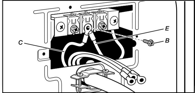
Connect neutral ground wire (E) and neutral wire (white) (C) of power supply cord under center terminal block screw (B). Tighten screw.
