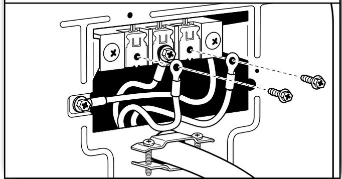
Connect remaining wires to outer terminal block screws. Tighten screws. Finally, reinsert tab of terminal block cover into slot of dryer rear panel. Secure cover with hold-down screw. Now, go to "Venting Requirements."
