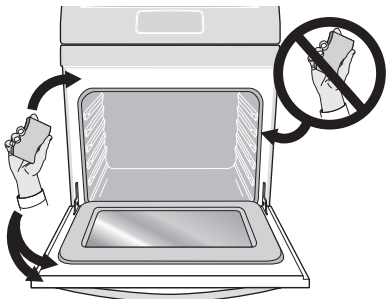
Figure 20: Clean around the oven door gasket
