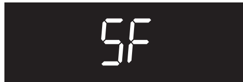
Figure 30: Display showing Sabbath failure
