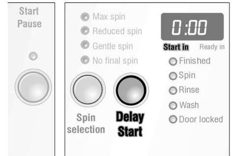
Press **Delay Start** button. The display shows the start time **0:00**.
