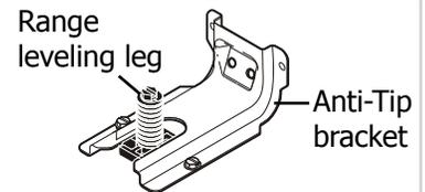
To check if the anti-tip bracket is installed properly, use both arms and grasp the rear edge of range back. Carefully attempt to tilt range forward. When properly installed, the range should not tilt forward.
