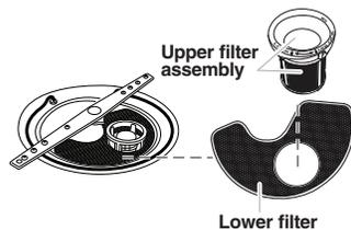
**IMPORTANT:** To avoid damage to dishwasher, do not operate your dishwasher without filters properly installed. Be sure lower filter is securely in place and upper filter assembly is locked into place. If upper assembly turns freely, it is not locked into place.
