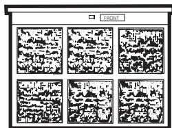
Dirty filter— Needs cleaning
