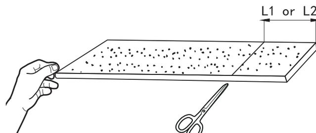
C Remove adhesive from back of foam insulation. Stick the foam insulation onto the left and right accordion, and inside of the frames.
