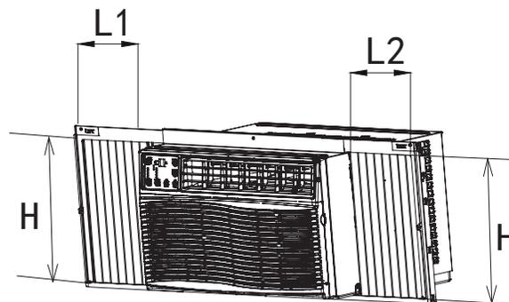
B Cut the foam insulation to the measured length of the left and right side accordion.
