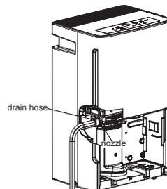
3. Thread a garden hose (not supplied) onto the nozzle, cut to length, and lead it to the floor drain.
