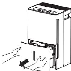
**IMPORTANT:** Do not use the hose if using the bucket to collect water. When the hose is connected, water will flow through it onto the floor instead of into the bucket.
