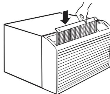
**NOTICE:** Do not operate the air conditioner without the filter in place. If a filter becomes torn or damaged it should be replaced immediately.
