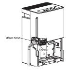
3. Thread a garden hose (not supplied) onto the nozzle, cut to length, and lead it to the floor drain.
