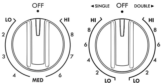
Figure 7: Single (L) and dual (R) radiant elements
