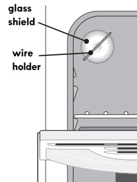
Figure 42: Replacing the oven light
