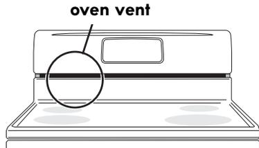
Figure 2: Do not block oven vent location
