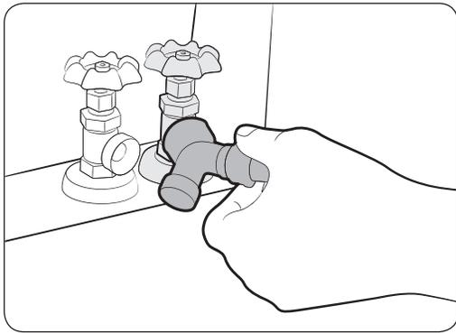
1. Close the cold water tap. If you have a washer cold water hose attached to the cold water faucet, unscrew and remove the hose. Then, connect the female end of the Y connector to the cold water tap.
