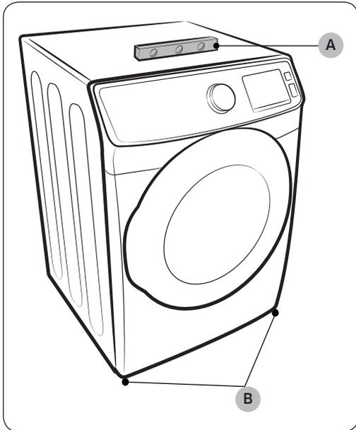
1. Using a **level (A)**, check if the dryer is level side to side and then front to back. If the dryer is not level, adjust the **leveling feet (B)** at the bottom of the dryer. Then, check if the dryer is level again.
