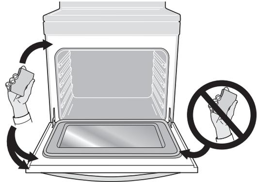
**Figure 9: Care in cleaning oven by hand**
