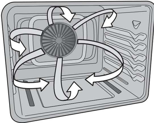
Figure 7: Air circulation in the convection function
