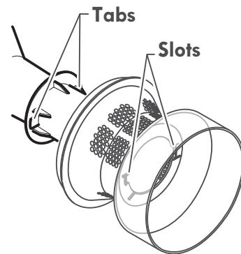
2. Rotate pre-filter clockwise to lock in place.
