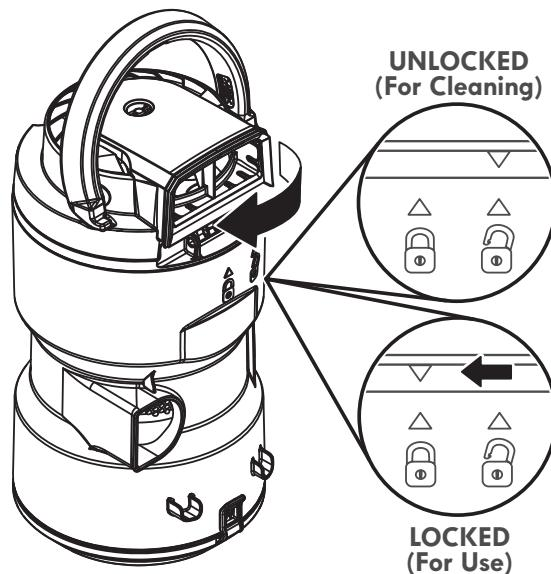
4. Rotate while pressing downward until marks align as shown; **LOCKED (For Use)**.
