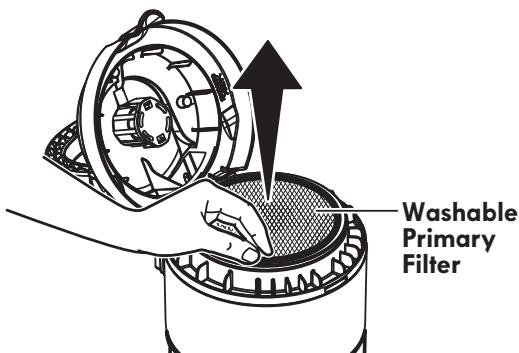
4. Wash with cold water only, **DO NOT** use detergent or soap. squeeze by hand and allow to air dry. Allow parts to dry 24 hours before putting back into vacuum cleaner.
