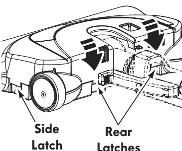
4. Rotate cover back. Press cover firmly until side and rear latches snap into place.
