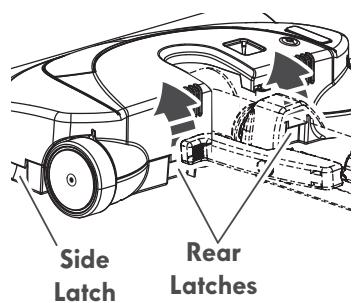
4. To remove cover, grasp the sides and pull out.
