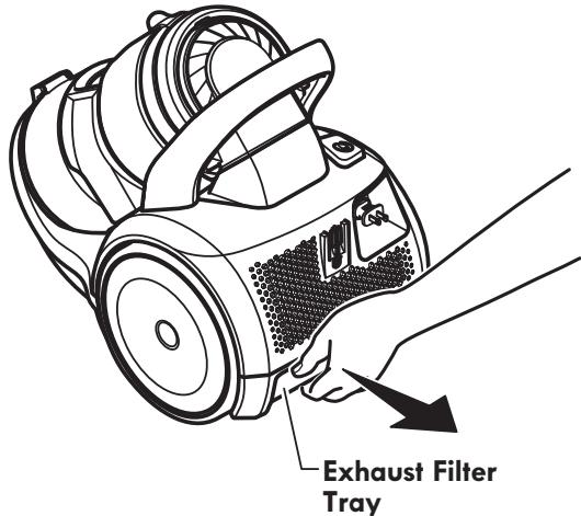
2. Remove exhaust filter from filter tray and dispose.
