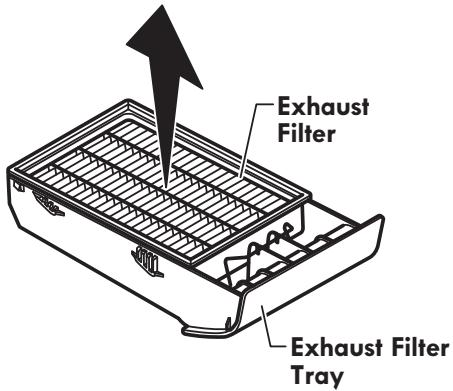
3. Replace exhaust filter cartridge. Place the new filter cartridge into the exhaust filter tray as shown.
