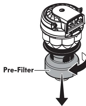
If necessary, rinse with cold water only, **DO NOT** use detergent or soap. Allow parts to dry 24 hours before putting back into vacuum cleaner.
