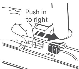
3. To replace the light bulb, carefully insert fully into slot.
