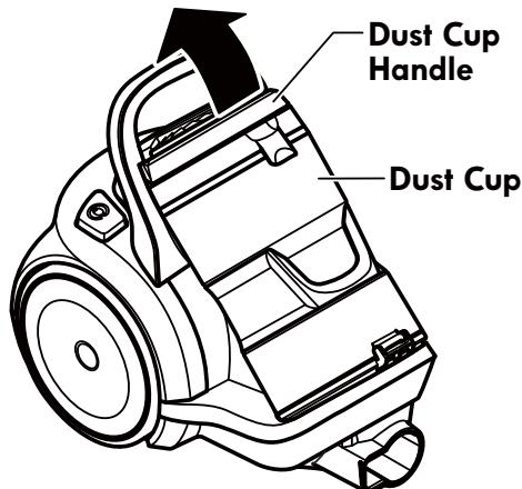
3. Pull the handle up and lift dust cup up and out of the vacuum cleaner.
