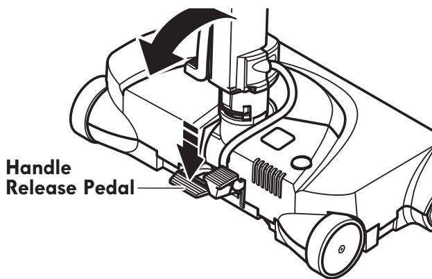
**4. Select a pile height setting by pressing the small pedal on the rear of the PowerMate®. The pile height setting shows on the indicator.**
