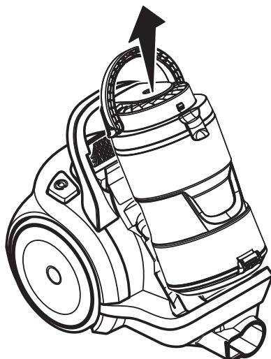
4. Remove any clogs that might be located in the suction port or filter port area.
