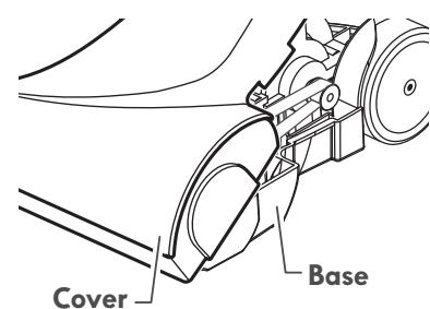
3. Line up front of cover and base. Rest cover on front edge of base as shown.
