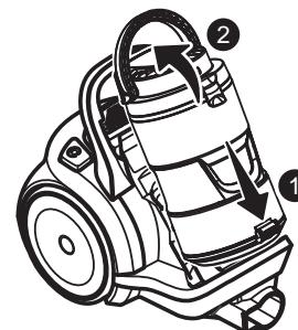
1. Place dust cup back into vacuum cleaner by inserting the bottom first and tilting back with the dust cup handle raised.
