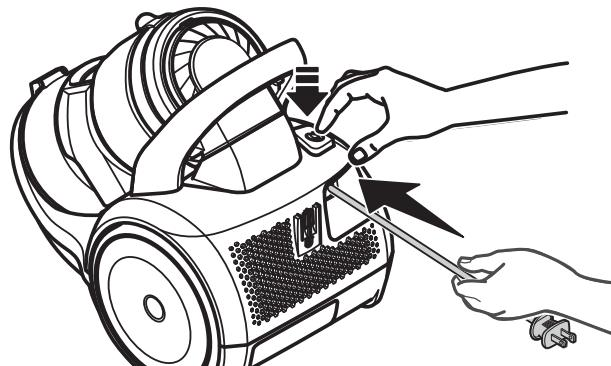
**3. Lower handle from upright position by pressing on the handle release pedal.**
