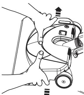
5. Lift agitator assembly out and remove worn belt.
