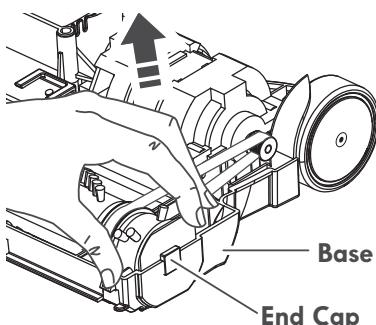
6. Check and clean end cap areas. See TO CLEAN AGITATOR (page 22) section and AGITATOR ASSEMBLY illustration (page 22) for picture of complete agitator assembly.
