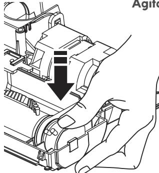
2. Push agitator assembly back into PowerMate®.
