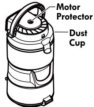
**To correct problem:** Empty the dust cup and clean the primary filter and pre-filter. Check for and remove clogs, and empty dust cup if necessary. See **REMOVING CLOGS** (page 16).
