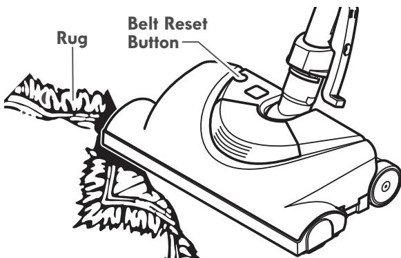
**To correct problem:** Turn off and unplug vacuum cleaner, remove obstruction, then press **BELT RESET** button.
