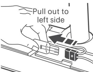
2. Remove the light bulb by pulling straight out.
