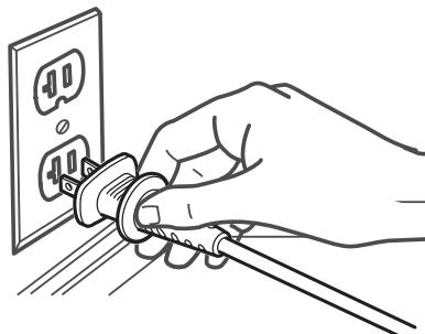
**NOTE:** To reduce the risk of electric shock, this vacuum cleaner has a polarized plug; one blade is wider than the other. This plug will fit in a polarized outlet only one way. If the plug does not fit fully in the outlet, reverse the plug. If it still does not fit, contact a qualified electrician to install the proper outlet. Do not change the plug in any way.
