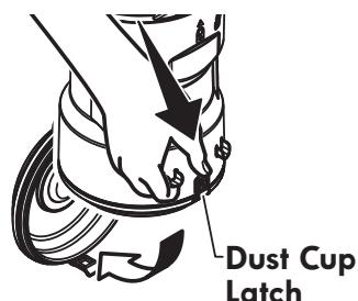
3. Press the dust cup latch slightly outwards and downward to release the door.
