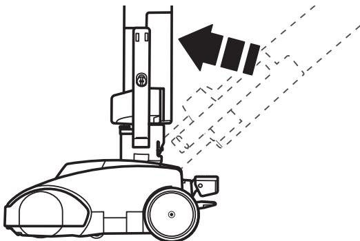
2. Press wand quick release pedal with foot and pull the telescoping wand straight up and out of PowerMate®.
