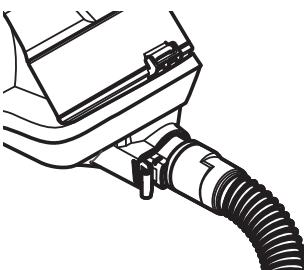
The hose swivel allows the hose to turn without moving the canister. This is helpful for cleaning in small areas.
