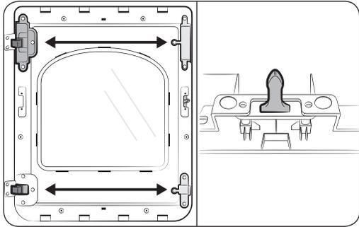
7. Remove the glass holder, and switch the positions of:
