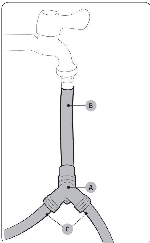
1. Close the cold water tap. If you have a washer cold water hose attached to the cold water faucet, unscrew and remove the hose. Then, connect the **short hose (B)** to the cold water tap. Turn the coupling manually until it is tight.
