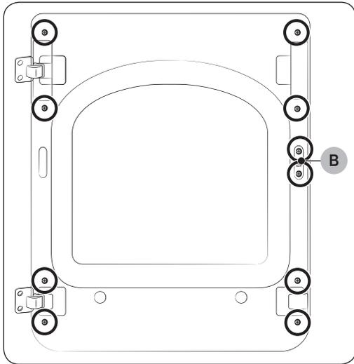
3. Remove the two screws from the lever holder, and then remove the holder cover.
