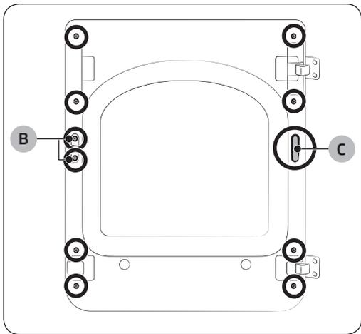
9. Remove the **hole cover (C)**, and then insert and tighten the glass holder using the removed 10 screws.
