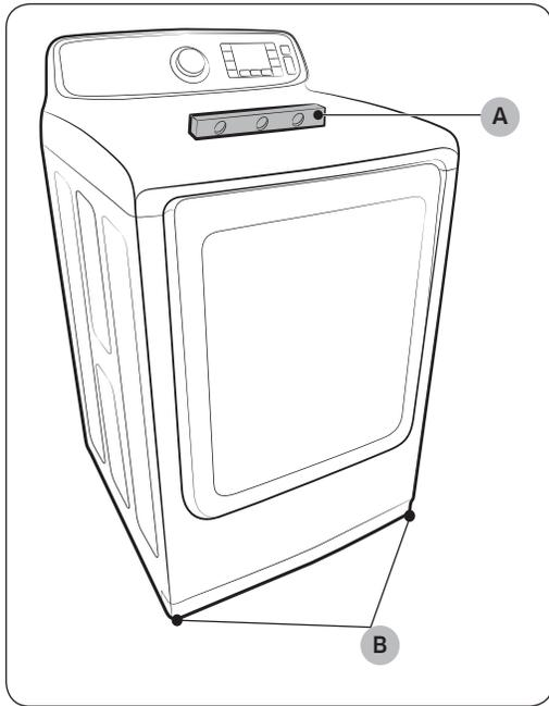
1. Using a **level (A)**, check if the dryer is level side to side and then front to back. If the dryer is not level, adjust the **leveling feet (B)** at the bottom of the dryer. Then, check if the dryer is level again.
