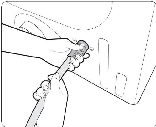
1. Close the cold water tap. If you have a washer cold water hose attached to the cold water faucet, unscrew and remove the hose. Then, connect the female end of the Y connector to the cold water tap.
