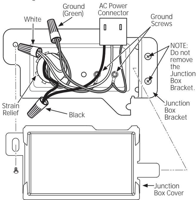
**NOTE:** All ground screws, brackets and wires must remain intact.
