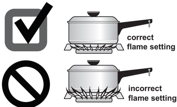
Figure 8: Correct and incorrect flame settings
