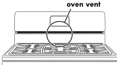
**Figure 9: Do not block oven vent location**
