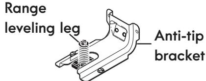
To check if the anti-tip bracket is installed properly, use both arms and grasp the rear edge of the range back. Carefully attempt to tilt range forward. When properly installed, the range should not tilt forward.
