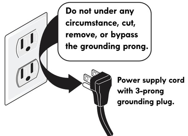
Figure 1: Grounding type wall receptacle
