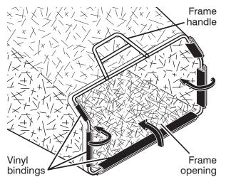
**ACAUTION:** Under normal usage, the catcher material is subject to deterioration and wear and should, therefore, be checked frequently for replacement. Any replacement catcher should be checked to ensure compliance with original manufacturer's specifications.
