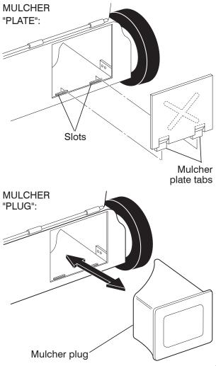
MULCHER PLUG BUILT INTO REAR DOOR
