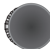
Incorrect Burner Cap Placement
