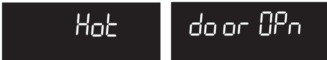
Figure 51: Hot message showing oven door locked (L) door OPn message will flash while door is opening
