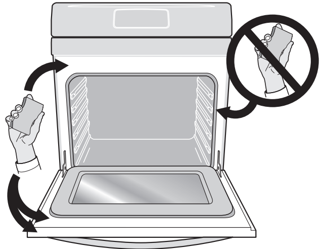
Figure 49: Oven door area to clean and not clean (gasket).
