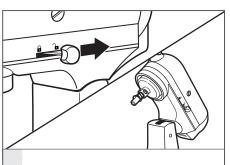
Hold the locking lever in the UNLOCK position and tilt motor head back. 2
