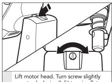
2 Int motor nead. Turn screw signtly counterclockwise (left) to raise flat beater or clockwise (right) to lower flat beater. Make adjustment with flat beater, so it just clears surface of bowl. If you over adjust the screw, the bowl lock lever may not lock into place.
