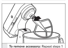
and 2. Press accessory upward as far as possible and turn to the 4 left. Then pull accessory from the beater shaft.
