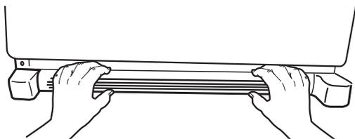
9. Using a  $\frac{3}{8}$ " hex wrench, remove the leveling leg brackets from the bottom of the cabinet. Keep screws for later use.
