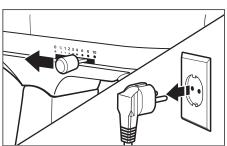
Turn Stand Mixer off and unplug before cleaning. Wipe the Stand Mixer body with a soft, damp cloth. Do not use household/commercial cleaners. Wipe off the beater shaft frequently to remove any accumulation of residue. Do not immerse in water.
