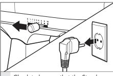
Check to be sure that the Stand Mixer is unplugged, and the speed control is turned to "0".
