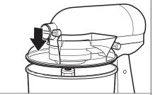
(OPTIONAL) Place the pouring shield\*: Slide the pouring shield\* from the front of the Stand Mixer over the bowl until the pouring shield\* is centred. The bottom rim of the pouring shield\* fits inside of the bowl. The pouring chute will be just to the right of the attachment hub as you face the Stand Mixer.
