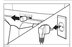
Check to be sure that the Stand Mixer is unplugged, and the speed control is turned to "0".
