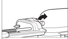
Tighten the attachment knob by turning it clockwise until the attachment is completely secured 4 to the Stand Mixer. See the Instructions manual that came with your attachment for detailed directions on using the attachment.
