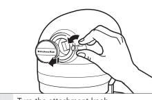
Turn the attachment knob counterclockwise to remove attachment hub cover.
