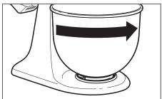
Remove the bowl: Gently turn the bowl counterclockwise to release it from the bowl clamping plate.
