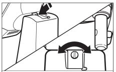
(OPTIONAL) To adjust beater to bowl clearance: Tilt the motor head back: then turn the screw slightly counterclockwise (left) to raise the beater, or clockwise (right) to lower the beater. Adjust the beater so that it just clears the surface of the bowl. If you over adjust the screw, the bowl lock lever may not lock into place.
