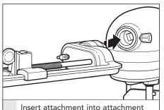
hub, making certain that attachment power shaft fits into the square attachment hub socket. It may be 3 necessary to rotate the attachment back and forth. When it is in the proper position, the pin on the attachment will fit into the notch on the hub rim.
