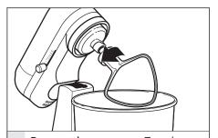
Remove the accessory: Turn the speed control to "0", unplug the Stand Mixer, and tilt the motor head 2 back; then, press the accessory upward as far as possible, then turn the accessory clockwise and pull it away from the beater shaft.
