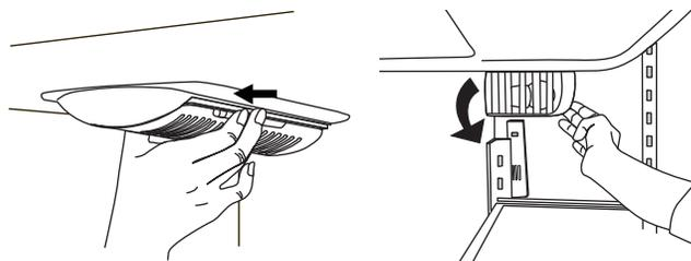
3. Replace the burned-out LED bulb(s) with a bulb of the same size, shape and wattage.
