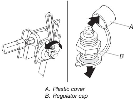
3. Flip the regulator cap over and replace the plastic cover.
