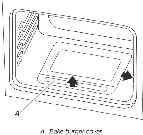
4. Lift up and remove oven bake burner cover.
