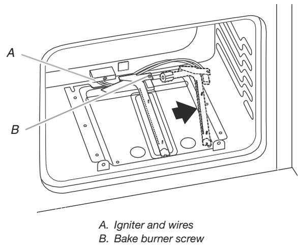
8. Unscrew and remove the cover over the orifice.
