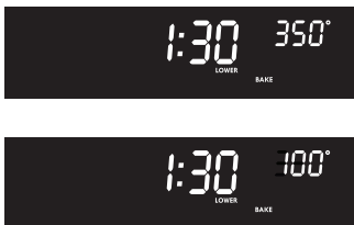
Figure 24: Set temperature shown (top). Minimum temperature appears when oven is started (below)
