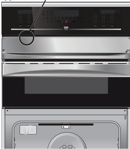
Figure 16: Oven vent location
