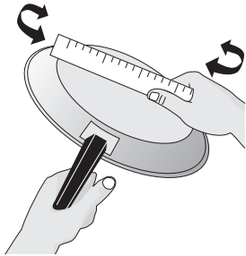
Figure 2: Check pan for flat bottom using ruler
