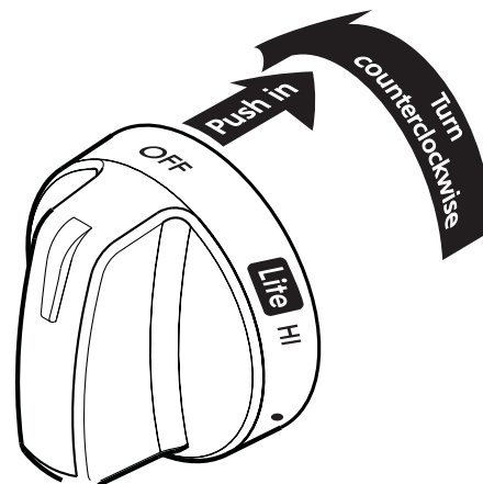
Figure 8: Proper way to set burners
