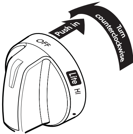
Figure 9: Setting the double ring burner
