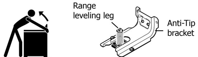
To check if the anti-tip bracket is installed properly, use both arms and grasp the rear edge of range back. Carefully attempt to tilt range forward. When properly installed, the range should not tilt forward.
