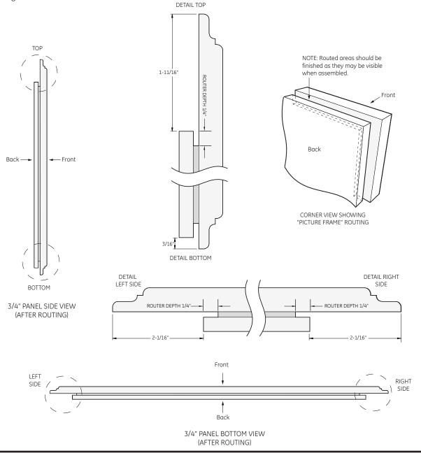
NOTE: For panels constructed with rails and stiles (5-panel), the minimum width is 3" for rails and 4" for stiles.
