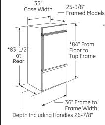
Shipping height. The refrigerator can be adjusted to fit into a cutout that is 85" max. height. Use leveling legs and wheels for a maximum 1" height adjustment.
