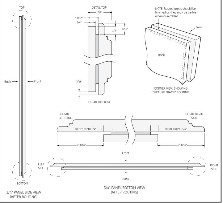
NOTE: For panels constructed with rails and stiles (5-panel), the minimum width is 3" for rails and 4" for stiles.
