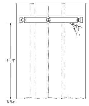
• Locate at least 2 studs on the back wall. Mark these points on the horizontal line.
