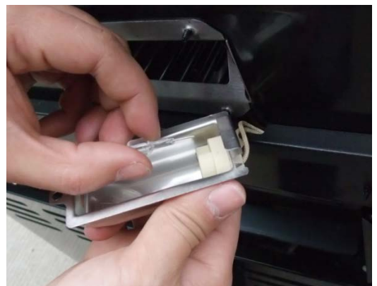
6. Wiggle the old bulb free from the bulb socket.
