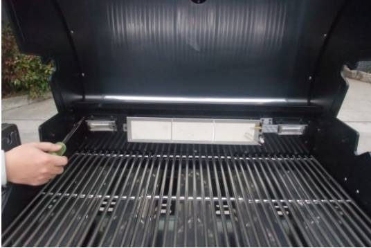
1. Remove the rear panel screws and nuts.
