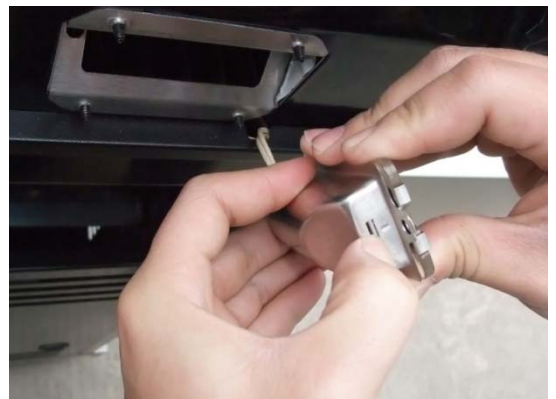
5. Press button on end of bulb case to free and remove bulb case glass.
