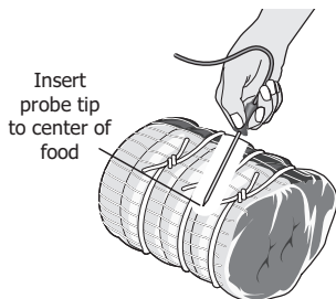
Figure 35: Proper probe placement
