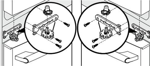
Once both doors are in place, ensure they are aligned with each other and level (Please see the "Installation" section for more details), and replace the top hinge cover.
