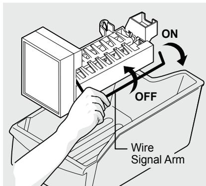
gain access to the ice maker, pull the freezer drawer out. Lift the wire signal arm to turn the ice maker OFF and lower the wire signal arm to turn it ON.
