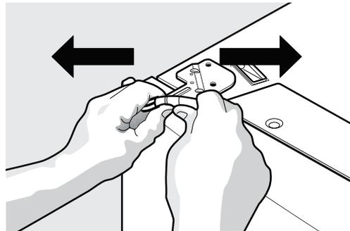
3. Detach the water tube from the connector located behind the refrigerator and pull the tube back out to the front of the unit. The connector releases when you press inward on the outer sleeve while pushing the tube toward the connector then while continuing to hold in the sleeve, pull the tube away.
