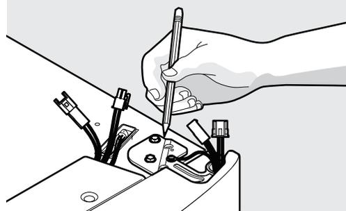
2. Disconnect the harness by grasping both sides of the connector firmly, depress the latch, and pull apart. Remove the two screws from the top hinge. Lift the door off of the bottom hinge and set it aside.
