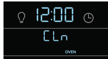
Figure 37: Clean lock icon blinks as door unlocks
