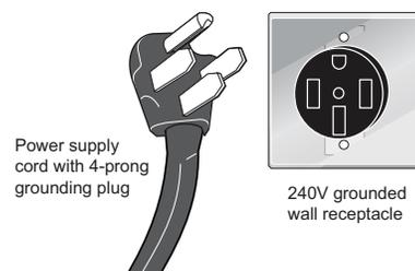
It is the personal responsibility of the consumer to have the appropriate outlet with the correct, properly grounded wall receptacle installed by a qualified electrician.
