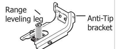
To check if the anti-tip bracket is installed properly, use both arms and grasp the rear edge of range back. Carefully attempt to tilt range forward. When properly installed, the range should not tilt forward.
