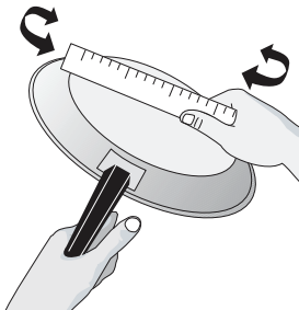
Figure 3: Checking the pan for flatness
