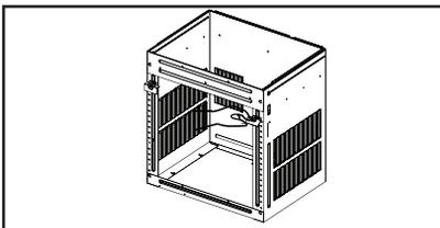
5. Insert the frame curtain into the upper guide and frame guides.
