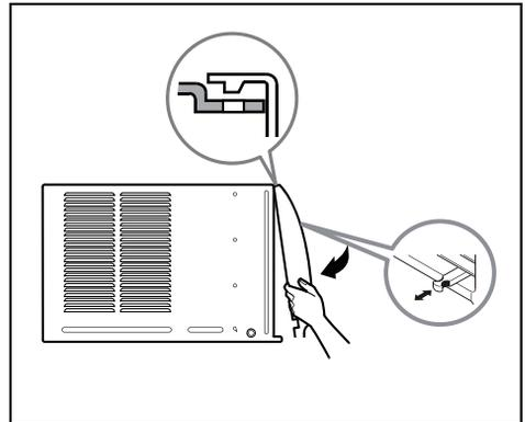
11. Put down inlet grille and take out the filter and secure it with 2 Type A screws through the front grille.
