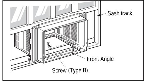
3. Pull each frame curtain fully to each window sash track, and pull the bottom window sash down behind the top retainer bar until it meets.
