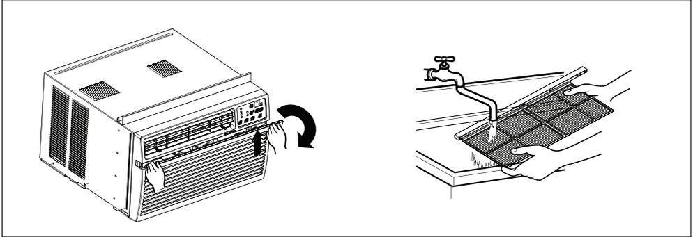
1. Remove the air filter from the front grille by pulling forward the air filter and then up slightly.
