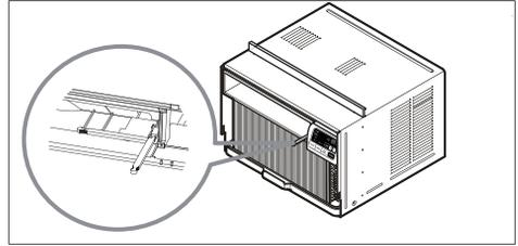
9. Cut the adhesive-backed Foam-Heatproofs to the Guide Panel size.
