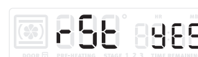
Figure 30: Display will show choice to reset to default (rSt yes) or to remain with user programmed options (rSt no)
