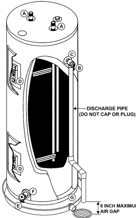
Never use this water heater unless it is completely full of water. To prevent damage to the tank and heating element, the tank must be filled with water. The water must flow from the hot water faucet before turning "ON" power.
