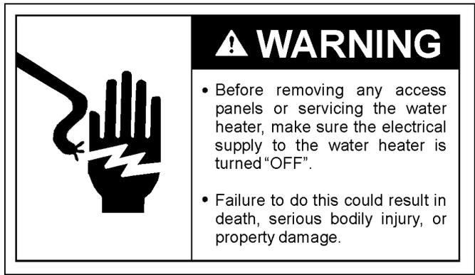
1. Before beginning, turn “OFF” electrical power supply to the water heater.
