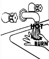
Water temperature over 125°F (52°C) can cause severe burns instantly resulting in severe injury or death.
