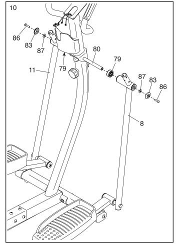
11. Remove and discard the packaging on the Right Crank Bracket (30). Then, tighten an M8 x 14mm Shoulder Screw (86) with a Pivot Cover (83) and an M8 Washer (87) into the right Crank Arm (24).
