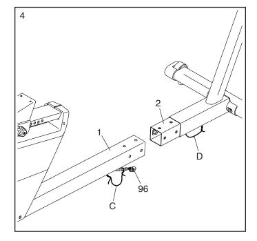
5. **Tip: Avoid pinching the wires.** Insert the Upright (2) into the Frame (1).
