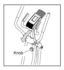
Next, lift a pedal, unfold the brace, and insert the end of the brace into the pedal arm. Make sure that the brace is securely inserted into the pedal arm. Repeat this action for the other pedal.
