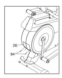
Next, locate the Reed Switch (60). Slightly loosen the two M4 x 16mm Screws (84).
