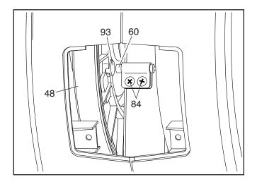
Next, rotate the Large Pulley (48) until a Pulley Magnet (93) is aligned with the Reed Switch (60). Slide the Reed Switch slightly toward or away from the Pulley Magnet. Then, retighten the M4 x 16mm Screws (84).
