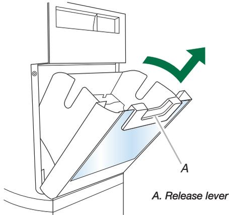
**NOTE:** It is not necessary to flip the ice maker On/Off switch to the OFF (down) position when removing the storage bin. The storage bin sensor, located on the right wall of the freezer door, stops the ice maker from producing ice if the door is open or the storage bin is removed.
