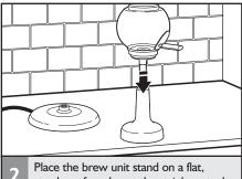
Place the brew unit stand on a flat, sturdy surface. Insert the stainless steel siphon tube into the brew unit stand.
