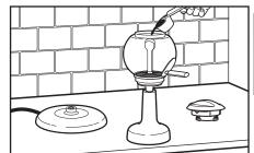
2 Scoop the desired amount of ground coffee into the brew unit using the coffee scoop; then, place the lid on the brew unit. See the "Dosage recommendation chart" on page 11 for more information.
