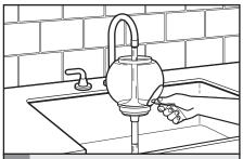
4 Hold the stainless steel siphon tube above a sink and remove the palm of your hand to empty the water and coffee grounds from the brew unit. Repeat steps 2 and 3 as needed.
