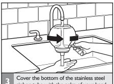
S siphon tube with the palm of your hand. Fill the brew unit with hot tap water, moving it in a circular motion to rinse away remaining coffee grounds.
