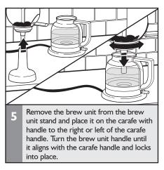
**NOTE:** The Siphon Coffee Brewer features a dual lock system that mechanically and magnetically locks the brew unit into place.
