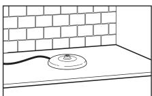
Place the base with power cord on a flat, sturdy surface and plug it into a grounded outlet. If desired, wrap excess cord around the cord holder on the bottom of the base.
