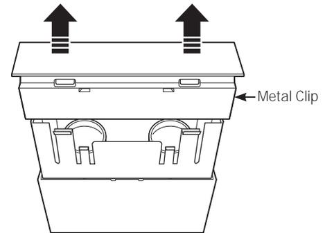
**WARNING** – The metal clip must be replaced or the heat from the bulb could damage the refrigerator.
