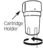
**NOTE:** A newly installed water filter cartridge may cause water to spurt from the dispenser.
