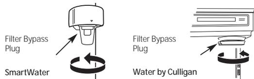
To use the filter bypass plug on Water by Culligan™ models, you must first remove the filter adaptor from the cartridge holder by turning it to the left.
