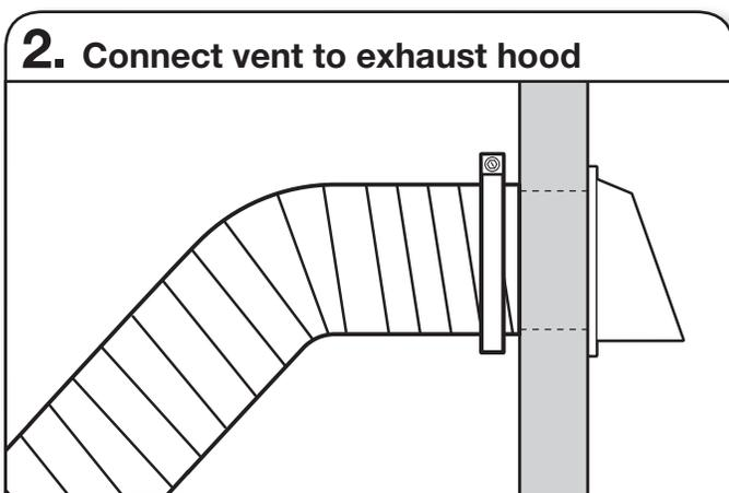
Vent must fit over the exhaust hood. Secure vent to exhaust hood with 4" (102 mm) clamp. Run vent to dryer location using straightest path possible. Avoid 90° turns. Use clamps to seal all joints. Do not use duct tape, screws, or other fastening devices that extend into interior of vent to secure vent, because they can catch lint.
