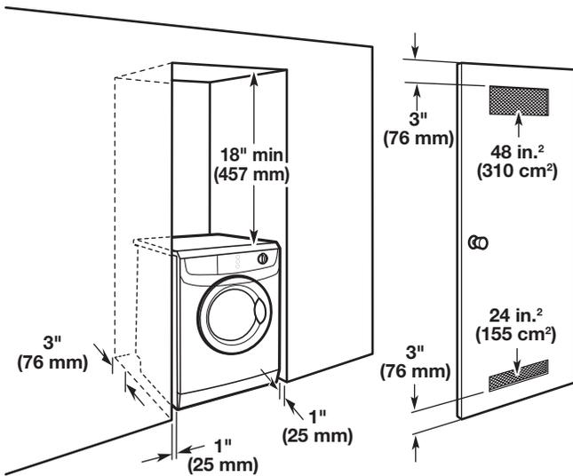
**Recessed or closet installation – Stacked with stack kit:**
