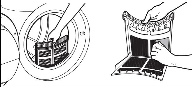
Clean the lint screen before each load. Pull the lint screen straight up. Open lint screen. Roll lint off the screen with your fingers. Do not rinse or wash screen to remove lint. Wet lint is hard to remove. Close lint screen. Push the lint screen firmly back into place.
