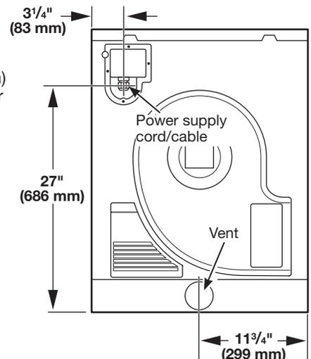
**Installation spacing for recessed area or closet installation**
