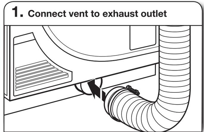
Using a 4" (102 mm) clamp, connect vent to exhaust outlet in dryer. If connecting to existing vent, make sure vent is clean. Dryer vent must fit over dryer exhaust outlet and inside exhaust hood. Check that vent is secured to exhaust hood with a 4" (102 mm) clamp.
