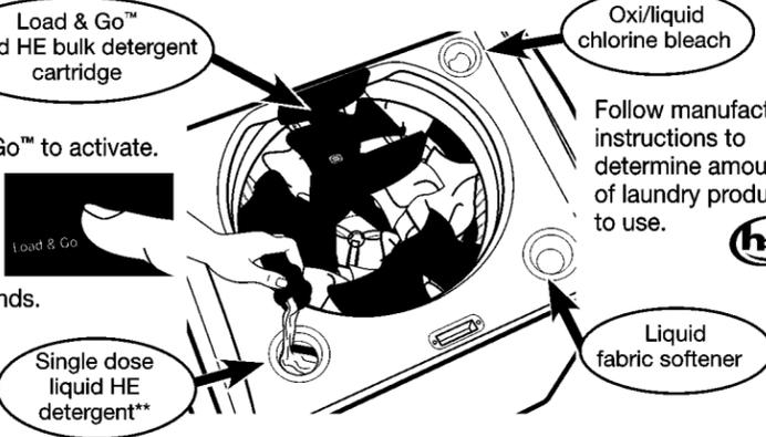
Load & Go™ liquid HE bulk detergent cartridge
